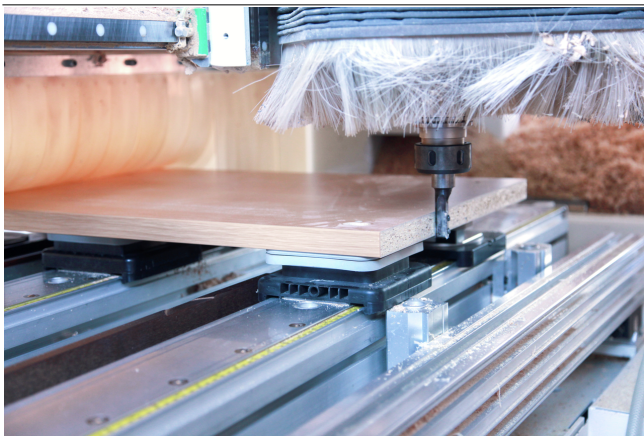
Vacuum blocks VCBL-S used with SCM consoles
